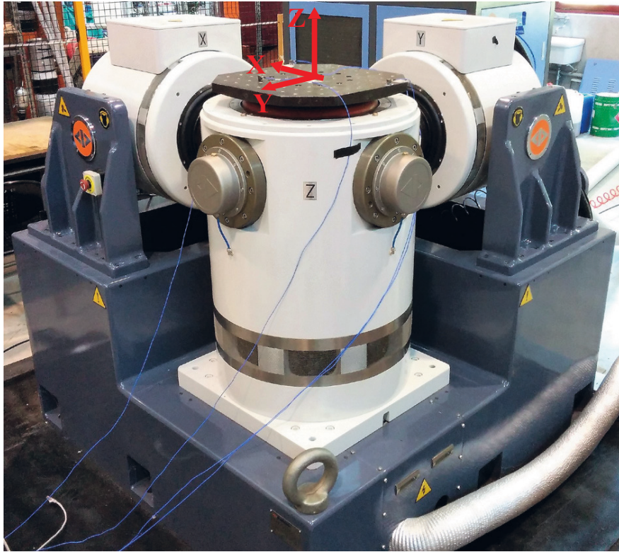
Figure 3: Three DoF shaker table at the University of Ferrara: Dongling 3ES-10-HF-500.
