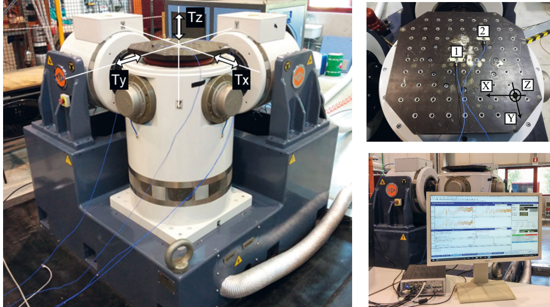
Figure 30: Test campaign setup: three-axial electrodynamic shaker at the University of Ferrara (left); bare head expander sensor configuration (right-top); Siemens SCADAS Mobile SCM202V (right-bottom).
