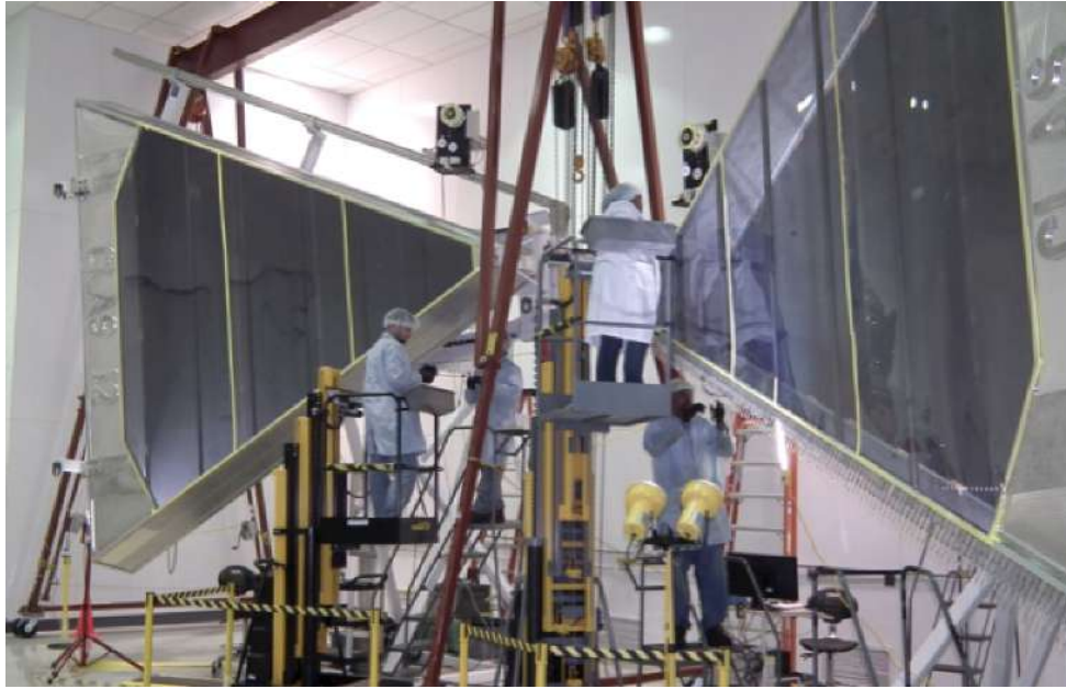
Figure 13: Simultaneous wire stringing of two R3 chambers in the Jefferson Lab clean room.
