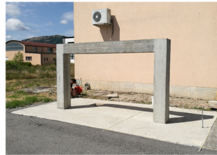
Figure 1. Sketch of the RC frame realized at the Hydrogeosite Laboratory (a,b): the structure is constituted by two columns (C1 and C2) and two beams (B1 and B2). Two different types of foundations are realized (F1 and F2). Photos of an intermediate constructive phase (c) and the final construction (d).
