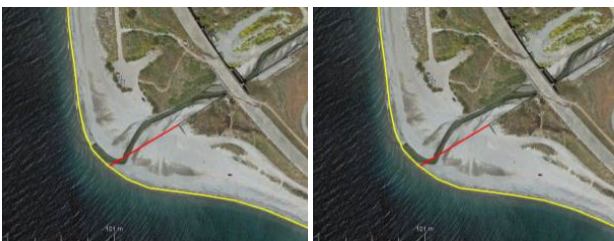
Figure 3. Maximum (to the left, in 2015) and minimum (to the right, in 2002) beach width. Legend: yellow = shoreline, red = transept. (source: satellite imagery of Google Earth Pro)
