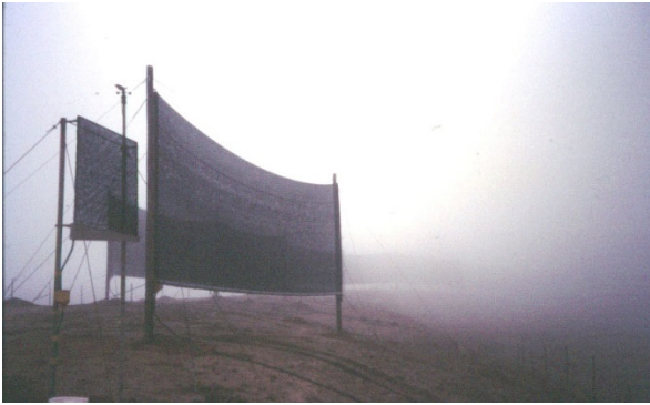
Figure 1. A Standard Fog Collector and a Large one in the Lomas the Mejia
