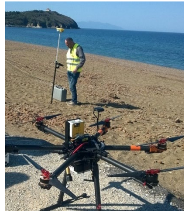
Figure 2. UAV equipped with MAIA multispectral camera used for the survey
