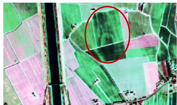
Figure 6. Radiometric enhance example. Contrast Stretching – Histogram Equalization on Pleiades image (ASTRIUM).
