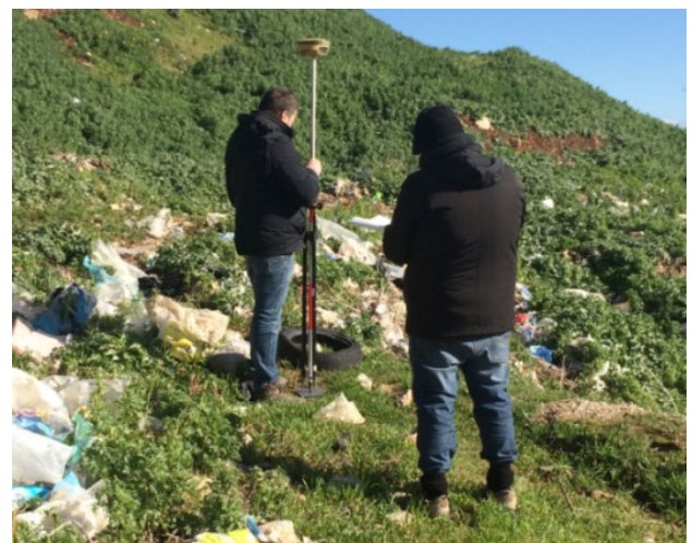
Figure 7. GNSS survey of the aluminium targets.
