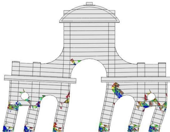
Figura 120: Crack pattern allo SLV
