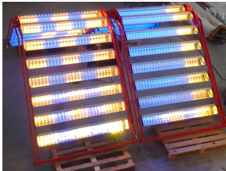
Fig. 6.3.2: The CPV modules are a linear low concentration parabolic concentrator which, in addition to a (daylight) energy production function, may perform nighttime functions as direct and/or diffused lighting, monochromatic and/or colored lighting
