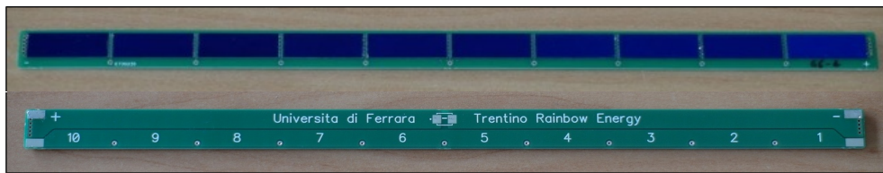
Fig. 5.2.2: In order to minimize the alignment errors, the cells are soldered onto a printed circuit board in series of 10. For each one of the cells are present test points so them can be tested individually.
