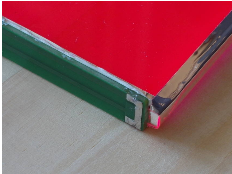
Fig. 2.2: A detail showing the edge of an LSC slab fitted with the receivers and the reflective film on the side edges, later an aluminium profile filled with silicone sealant have been installed around the receivers in order to protect the cells and the electrical connections from water and dust.
