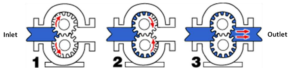
Figure 3. Cross section of external gear pump and the main working phases( http://www.pumpschool.com/principles/external.asp ).
