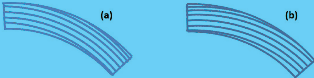
Figure 2.1: Schematic (not to scale) of the application of crystal for beam steering. The impact parameter b and the impinging angle of beam b' are shown. The surface roughness R_a of the lateral face of the crystal (parallel to beam direction) is required to be lower than the impact parameter b ( \sim 100 nm for beam halo of LHC) for beam steering using the channeling effect.
