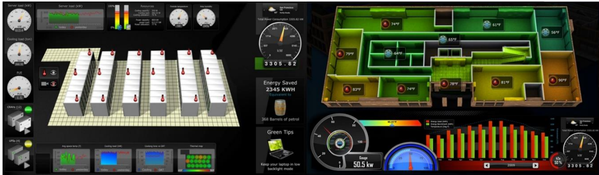
Figure 3.16: Examples of building automation systems visualization [121].
