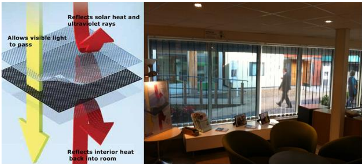
Figure 7.22: Illustration of In-flector insulators in the Building Research Establishment (BRE), Innovation Park Watford, UK [259].
