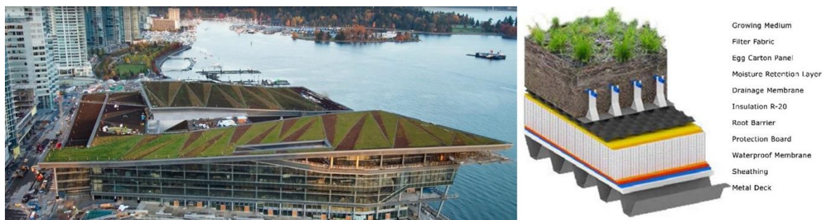
Figure 3.11: An example of a green roof project (left) and its detail (right) [103].
