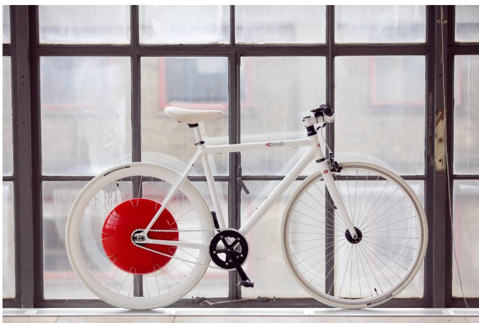
Figure 4.10: Copenhagen Wheel developed by MIT Senseable City Lab [151].
