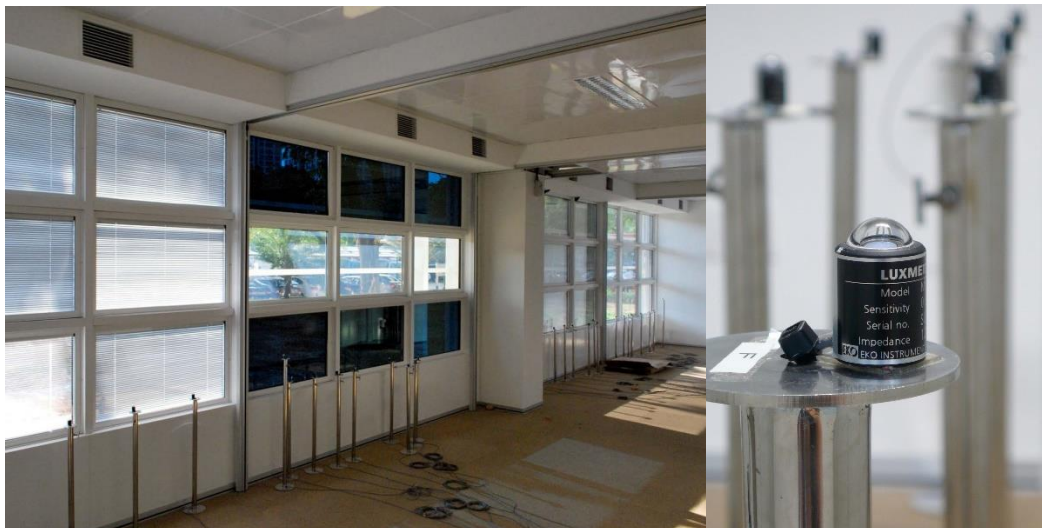
Figure 3.10: Façade equipped with four types from left to right: glazing integrated blinds, electrochromatic glazing, aSi photovoltaic glazing, and clear glass [99].
