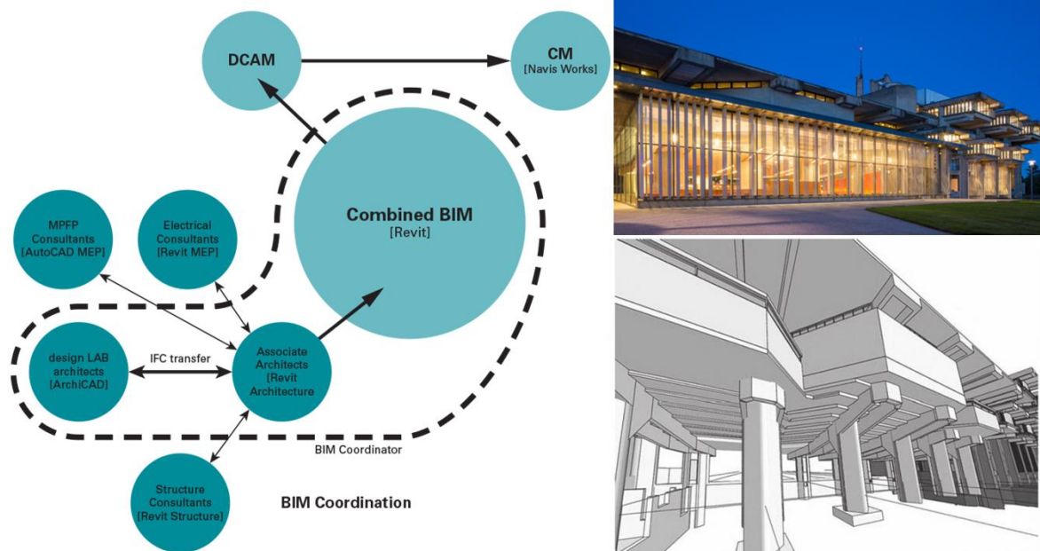
Figure 4.26: BIM implementation plan work flow diagram (left), west façade (top right) and existing conditions building model (bottom right) of Claire T. Carney Library, USA [188].
