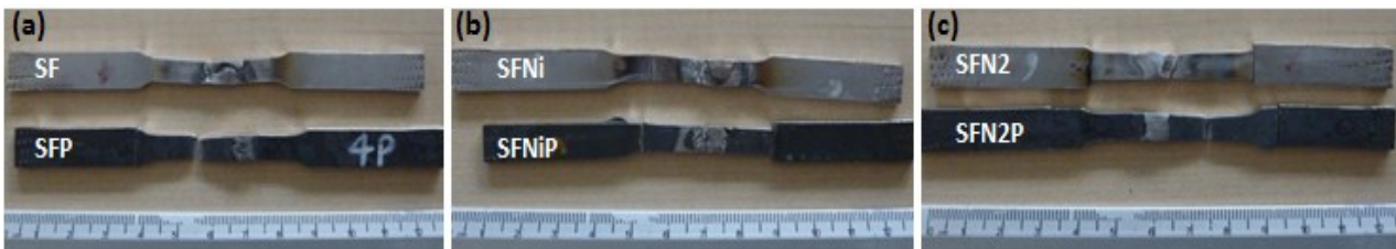
Fig. 2-50. Macro images of complete broken samples (a) SF, SFP (b) SFNi, SFNiP (c) SFN2, SFN2P
