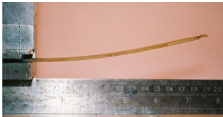
Figure 1.12 – Actuated E-glass/epoxy beam (Zhou and Lloyd, 2009)
