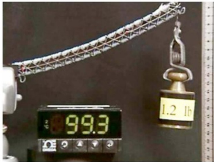
Figure 1.24 – A light weight SMA actuated truss beam (Sofla et al. , 2010)
