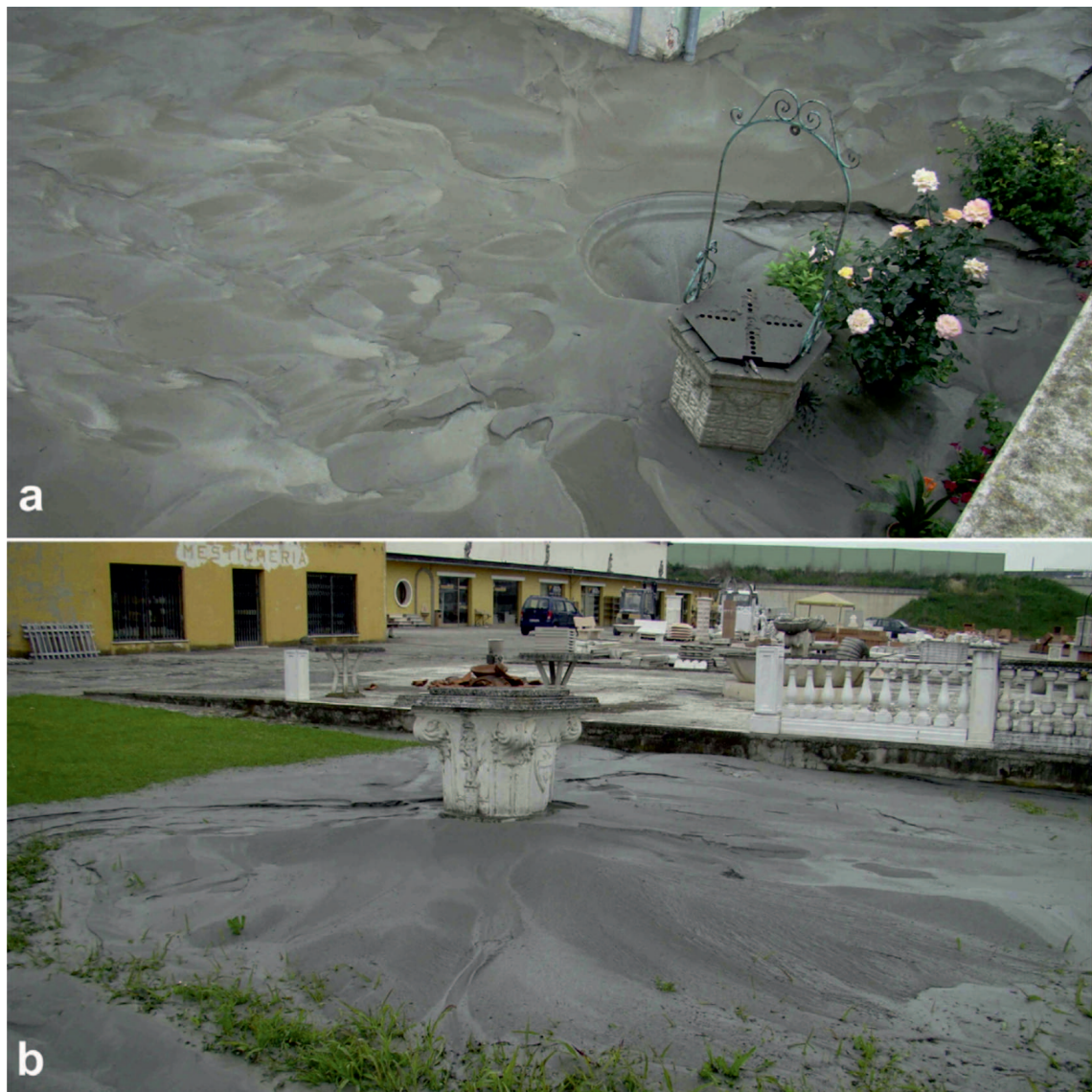
Figure 6.25: Examples of large-diameter water wells which locally enhanced the sand ejection during shaking and liquefaction of the sandy aquifer bodies (from Papathanassiou et al. , 2015).
