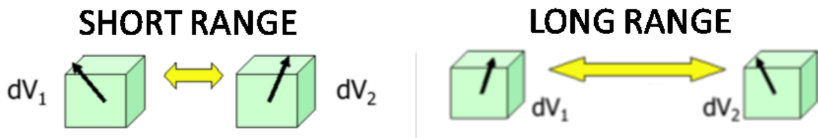
Fig. 1.3. Magnetic elements interacting by means of short range interaction and long range interaction.
