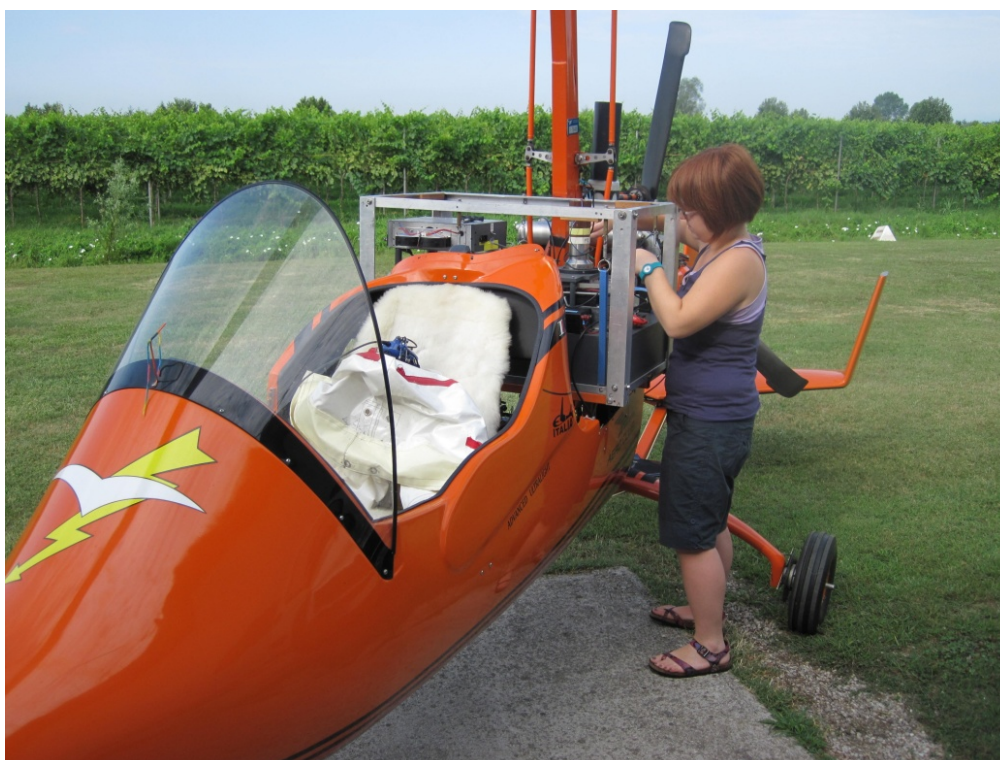
Figure 1.6 The AGRS_16L mounted on the autogyro used for the airborne \gamma -ray survey.
