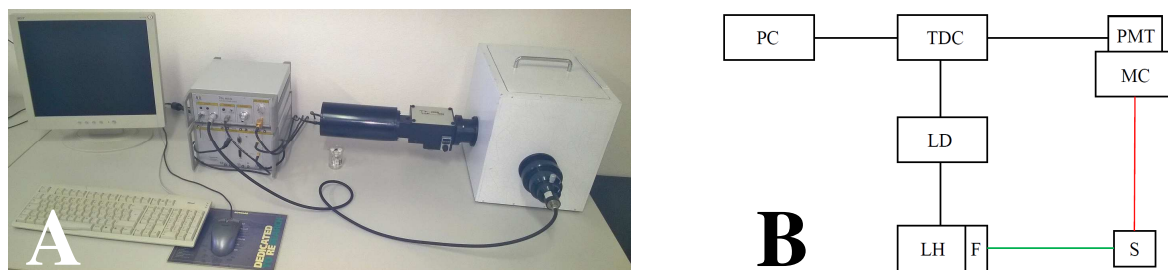
Figure 2.4 A) PicoQuant PicoHarp 300 TCSPC apparatus, used during this Ph.D. thesis. B) General scheme of a TCSPC apparatus: green line is the excitation beam; red line is the emission light; LH, laser head; F, filter; S, sample; MC, monochromator; PMT, photomultiplier tube; TDC, time-to-digital converter; LD, laser driver; PC, personal computer.
