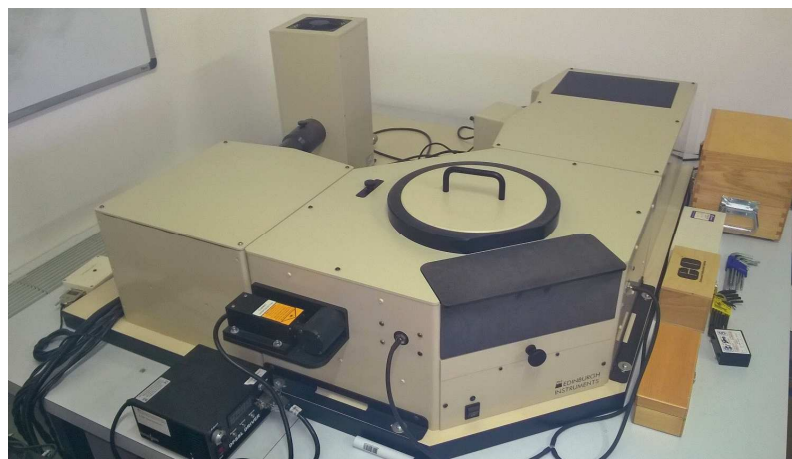
Figure 2.3 Edinburgh Instruments FLS 920 fluorescence spectrometer apparatus, used during this Ph.D. thesis.
