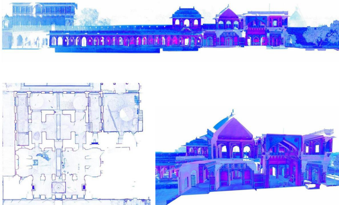
Fig. 5: Point cloud analyses at Nagaur Fort (credit: DIAPReM centre)
