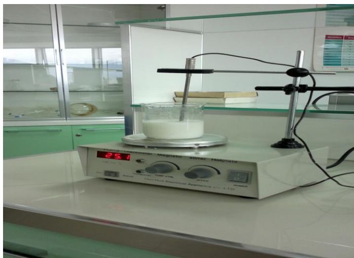
Figure 19. Magnetic stirring of mixture essential : \beta -cyclodextrine
