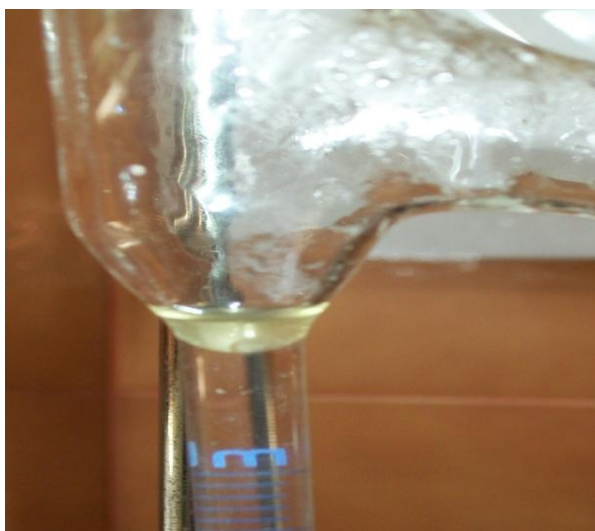
Figure 12. Essential oil extraction by Cleveneger
