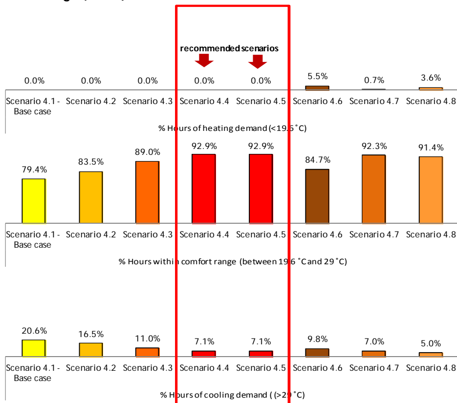
Figure 4.20 Effect of natural ventilation different scenarios on southern living room in typical floor during the month of October
