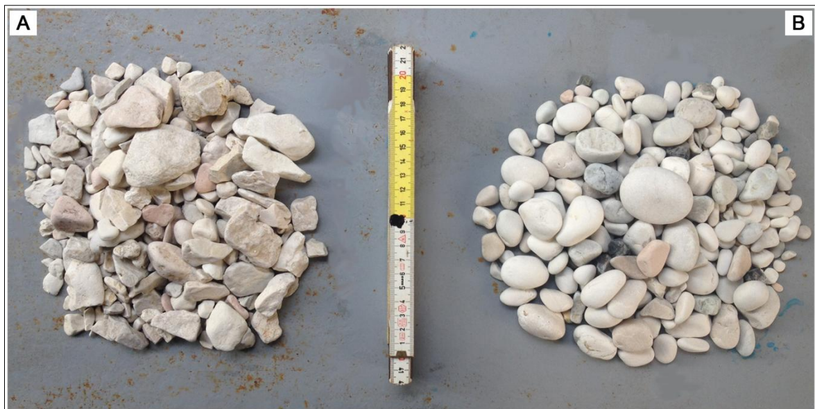
Figure 8-1- Comparison between a fill nourishment material adopted in Portonovo beach (A) and the native natural sediment (B).
