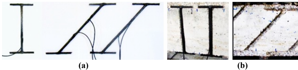
Fig. 2.32 Manually made FRP rods (MMFRP) proposed by (Jalali et al. 2012): (a) MM-NSM (b) groove prepared for the FRP installation.
