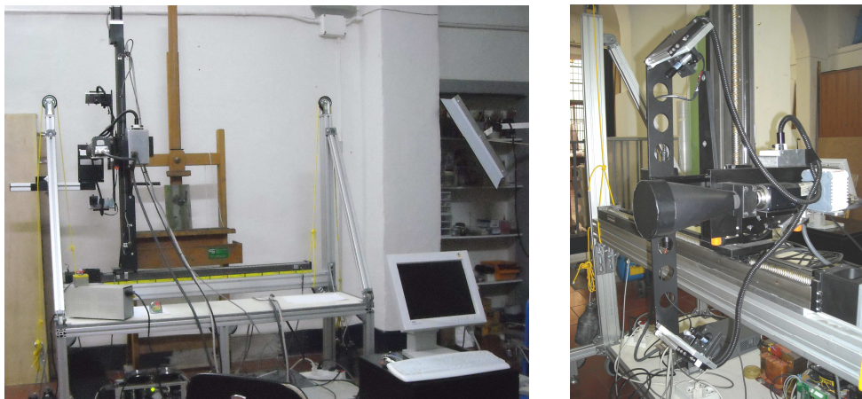
Figure 9 and Figure 10: Instrumental apparatus of the hyperspectral scanner; detail of the acquisition system .
