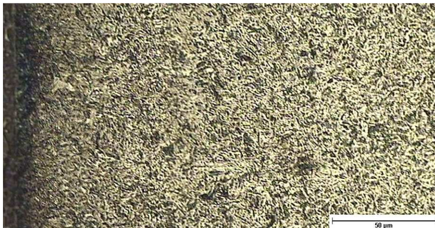
Figure 15 - Optical micrographs of a pin worn surface, when a 450 N normal load is applied in wet conditions.
