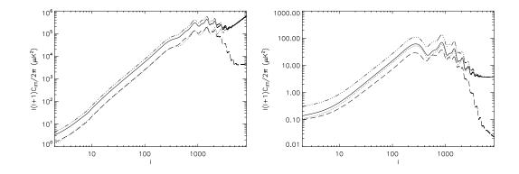
Figure 6.2: We computed the scalar power spectrum with the contribution of the Lorentz force-energy density cross correlation for  $n_B = 2$  (left panel) and  $n_B = -2.5$  (right panel). Solid line represents the correct assumption on the cross-correlation, the dotted line represents the result considering the Lorentz force and the energy density fully anti-correlated, triple dotted-dashed line represents the uncorrelated sum and the dashed line represents the result assuming full correlation.
