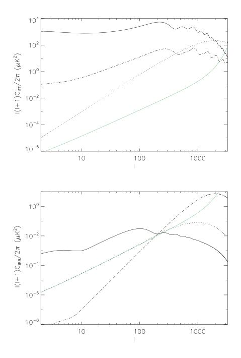
Figure 7.9: The noise level, beam convolved, for a 5' (green) CORE mission for temperature (upper panel) and B-mode polarization (lower panel), compared with primary CMB (black solid), magnetized vector mode (dotdashed) and magnetized scalar mode (dotted) or lensing (in the right panel) with  $B_{\lambda} = 6$ nG (with  $\lambda = 1$  Mpc) and  $n_B = -2.5$ .
