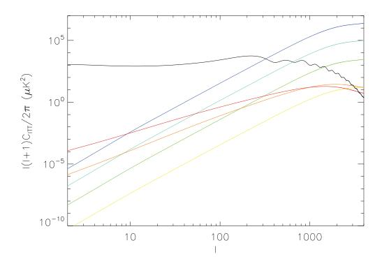
Figure 6.7: Temperature anisotropy angular power spectrum variation with the spectral index for the magnetized vector mode the amplitude of PMFs is fixed at  $B_{1\text{Mpc}}$  nG: black line is growing adiabatic scalar mode plotted for comparison, blue is  $n_B = 2$ , cyan is  $n_B = 1$ , green is  $n_B = 0$ , yellow is  $n_B = -1.5$ , orange is  $n_B = -2.5$ , red is  $n_B = -2.9$
