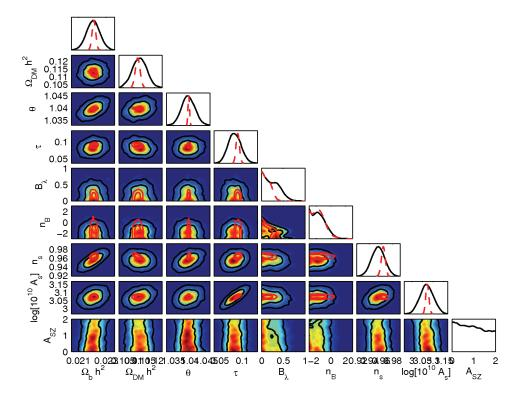
Figure 7.6: Triangle plot of the results of the comparison between the MCMC constrained with WMAP 7 years, ACBAR, BICEP and QUaD (black) and the one with *Planck* simulated data (red). Curves are the 68% and 95% confidence level.Note that  $B_{\lambda}$  (with  $\lambda = 1$  Mpc) is in 10 nG units.
