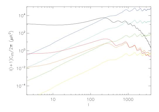
Figure 6.6: Temperature anisotropy angular power spectrum variation with the spectral index for the magnetized scalar mode the amplitude of PMFsis fixed at  $B_{1\text{Mpc}} = 6 \text{ nG}$ : black line is growing adiabatic mode, blue is  $n_B = 2$ , cyan is  $n_B = 1$ , green is  $n_B = 0$ , yellow is  $n_B = -1.5$ , orange is  $n_B = -2.5$ , red is  $n_B = -2.9$
