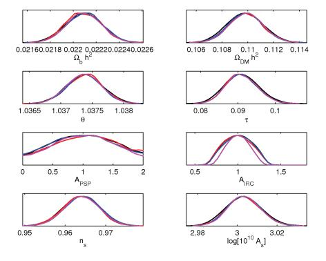
Figure 11.13: Comparison of the results of the MCMCs, with inverse noise variance weighting scheme, constrained with *Planck* simulated data with foreground and secondary anisotropy residual marginalization, for different frequency combinations. Black curve is 143 - 217 GHz, res curve is 100 - 217GHz, blues curve is 70 - 217 GHz and pink curve is 70 - 353 GHz.
