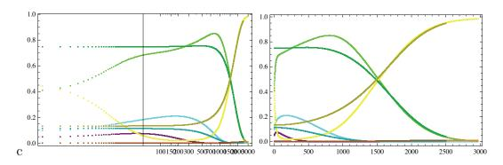
Figure 10.11: Noise plus foreground weights in lighter colors and inverse noise variance weights in darker colors lines on large scales (left panel) and small scales (right panel): purple and dark purple 70 GHz, cyan and dark cyan 100 GHz, green and dark green 143 GHz, yellow and dark yellow 217 GHz, orange and dark orange 353 GHz.
