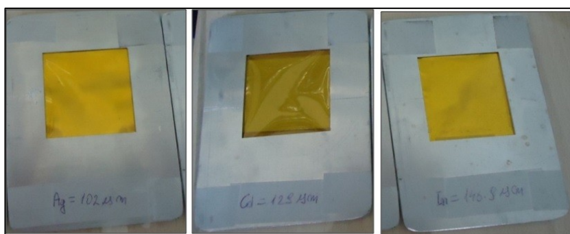
Figure 2.1 Filter foils Silver Ag, Cadmium (Cd), Indium (In).
