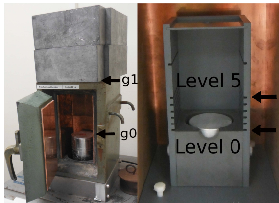
FIGURE 2.1: Photograph of the HPGe detectors used: on the right, Research detector (g0 and g1 geometries); on the left, Arrofixe detector (Level 0 and Level 5 geometries).
