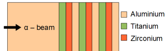
FIGURE 4.3: Scheme of a typical stacked target.
