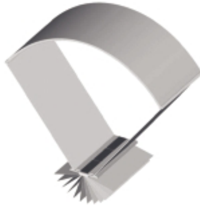
Figure 1.2 ENTECH mid-concentration photovoltaic module design using arched linear Fresnel lens [2]
