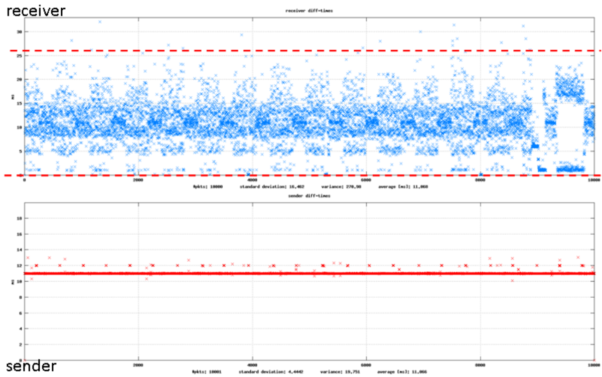
Figura 6.23: Worst case test - 1 stream - with FTP
