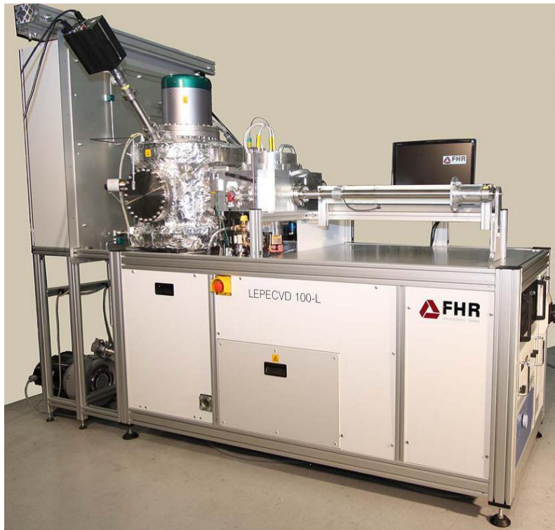
Figure 4.1: LEPECVD reactor in the clean room at SSL.
