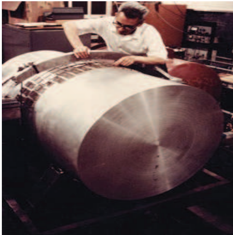
Figure 2.1: Joseph Weber working on the first resonant mass detector at the University of Maryland.
