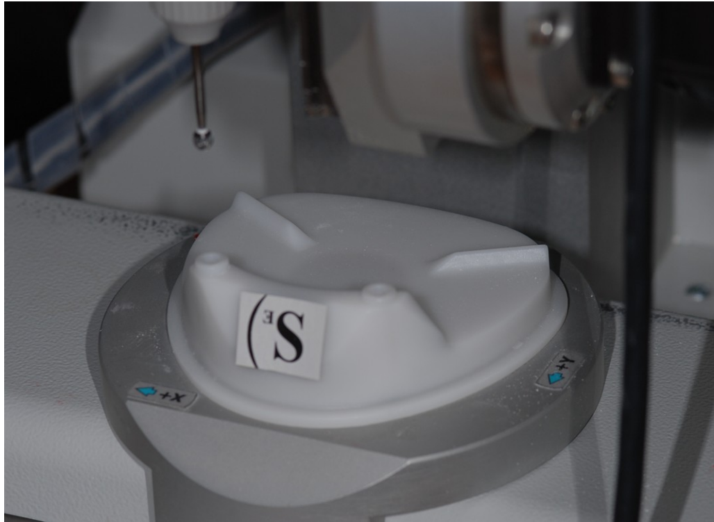
Fig. 6.5. Base interlocking system on the robot platform and robot axes directions
