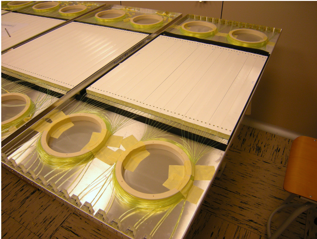
Figure 6.4: Internal view of an active layer.
