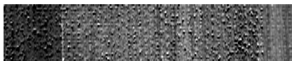
Figure 5.25: Mapping with SSD of Cadmium distribution: the Cd compound is on the right part of the sample
