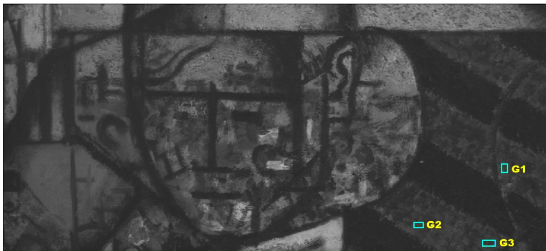
Fig. 4.43: J. Metzinger, At the Cycle-Race Track , PGC. Image acquired by IS at 530 nm, with measurements ROI on dark green areas G1, G2, G3.
