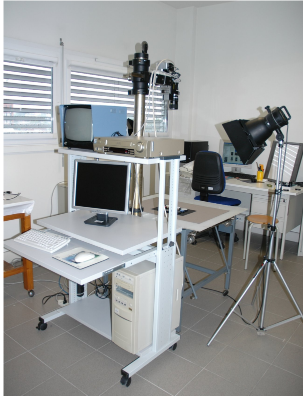
Fig. 1.6: Image spectroscopy apparatus, developed in the first years of 2000.
