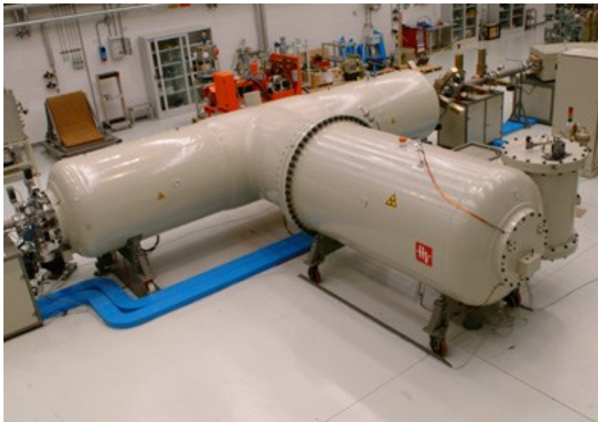
Fig. 2.7 Picture of the tank of the Tandem accelerator at LABEC.
