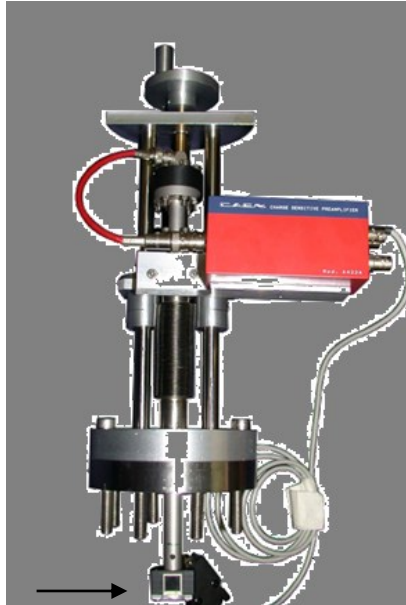
Fig 3.10 The new silicon detector (indicated by the black arrow) mounted on a retractable arm.
