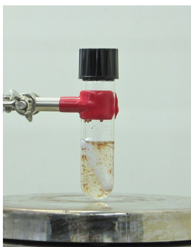
Fig 3.19 Picture of the oak sample during the bath in chloroform on the magnetic agitator.
