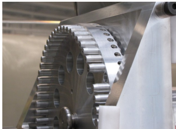
Fig 2.5 Picture of the wheel (“carrousel”) with graphite samples ready for the measurement.
