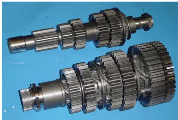
Figure 4.1 Gearbox including the gears analyzed [4.12].
