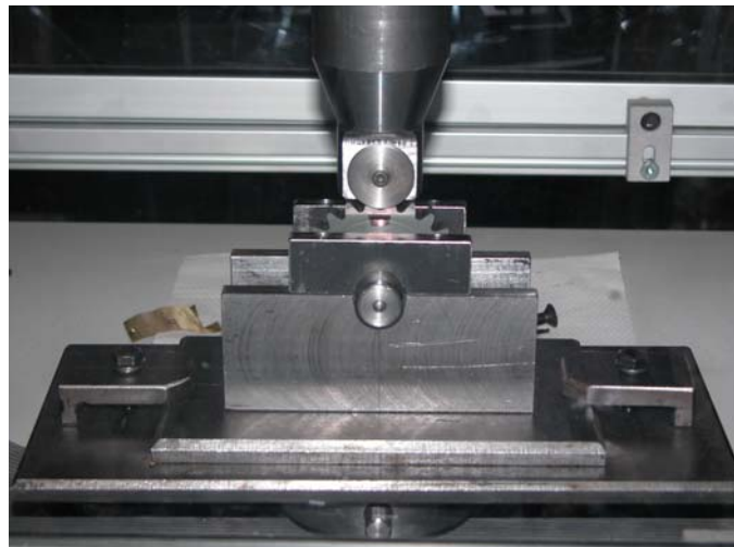
Figure 3.19 Picture of the device developed for bending and contact fatigue tests on spur gear teeth [3.51].
