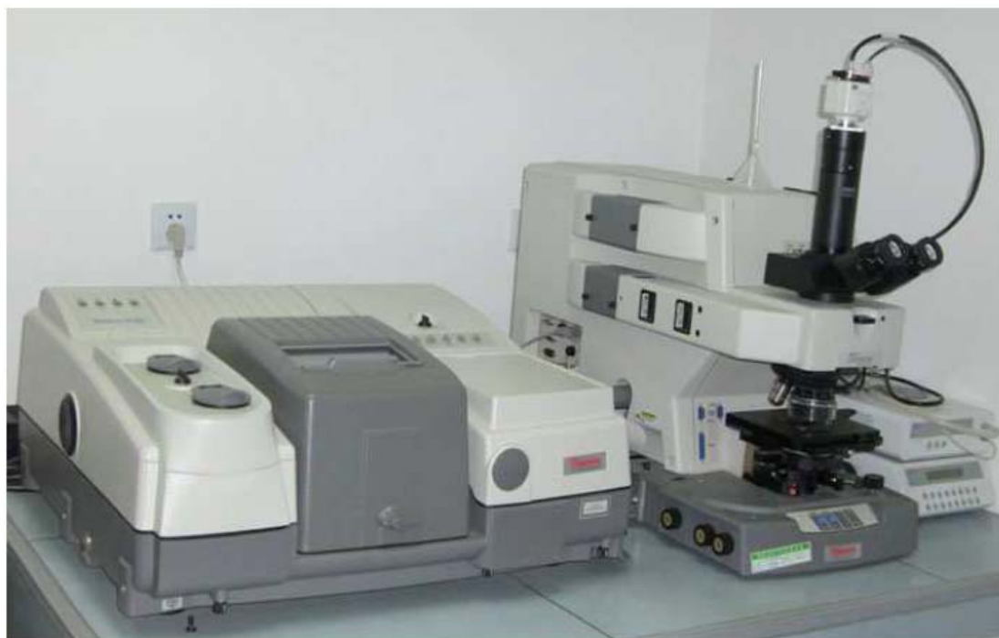
Fig. 3.1 - Picture of the Nicolet 5700 FTIR spectrometer coupled with a microscope
