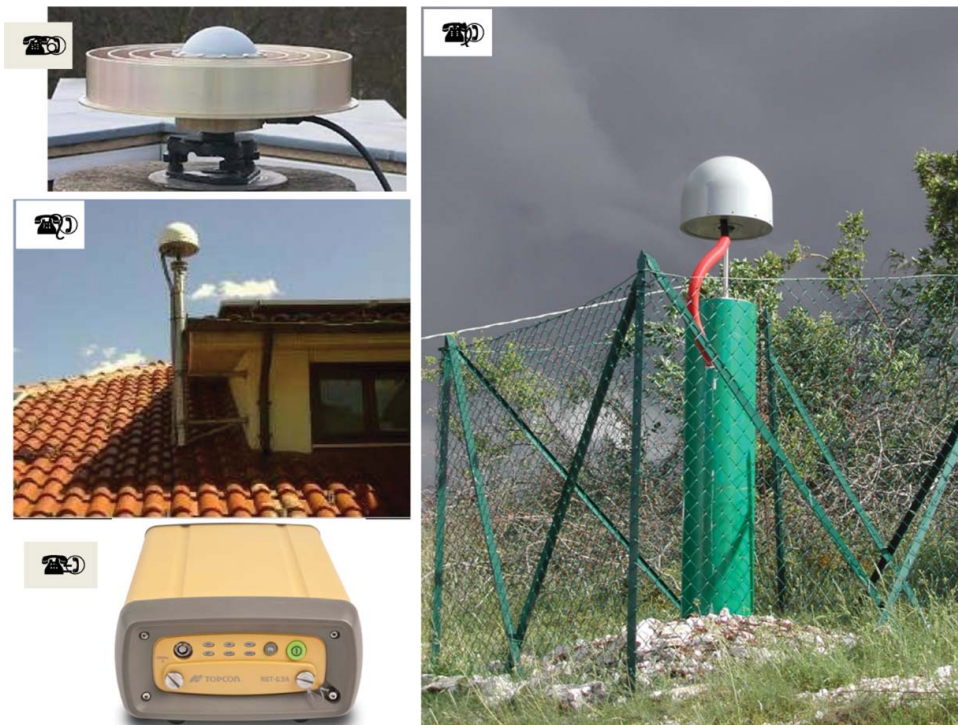
Figure 2. Choke ring antenna (a). Antenna on a building (b). Antenna on the ground (pillar) (c). GPS receiver (d).
