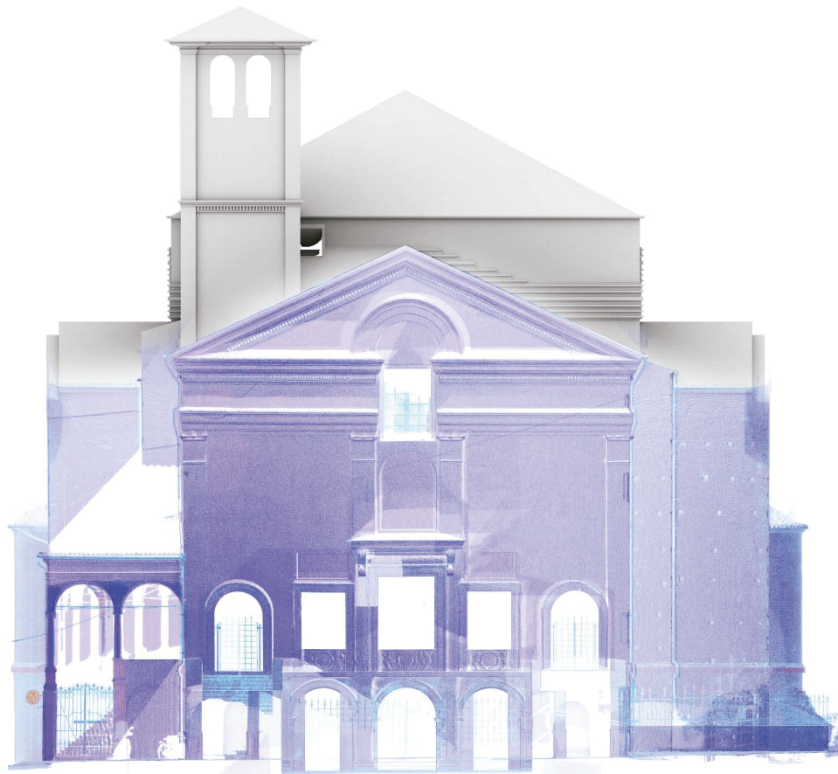
Fig 3. Tempio di San Sebastiano, Leon Battista Alberti, Mantua. Overlap between the point cloud obtained by means of 3D morphometric acquisition and its graphic rendering through BIM parametric modelling, and, in particular, Heritage-BIM environment
