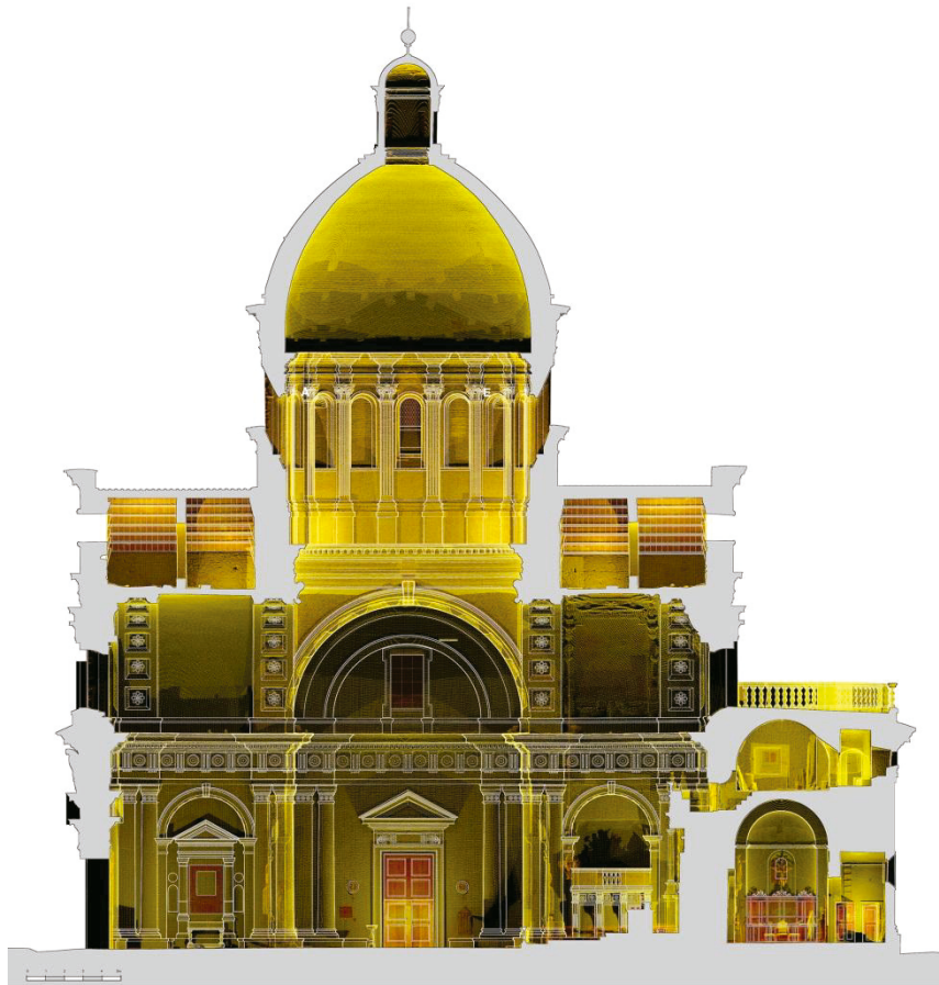
Fig 2. Cross section directly obtained from the point cloud model generated by the 3D integrated survey. The amount of information acquired, opportunely normalized (such as density and reflectivity index) allows analysis and direct interaction with the architecture, avoiding additional representation procedures. This acquisition-visualization method allows a high level of knowledge and usability of two-dimensional drawings reducing time and cost.
