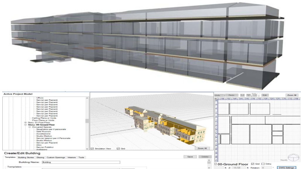
Fig6: Elaboration of the BIM relative to the pavilion of the San Luca. 3D zones and utilization of the model on a Simergy Pro interface platform for EnergyPlus. (Modeling source: L. Marzi - S. Leone- Becquerel Electric)
