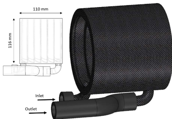
Figure 3. Water jacket to cool the electric motor
