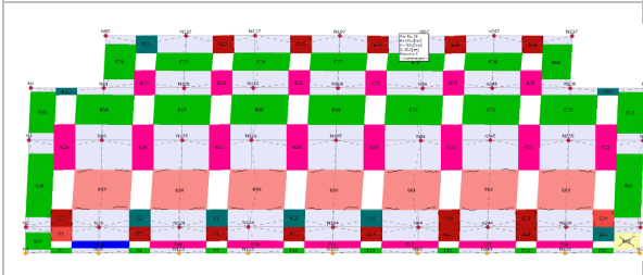
Analysis-12/Mechanism P.15 /2 nd Internal hall masonry /seismic dir.+X/seismic load =static
