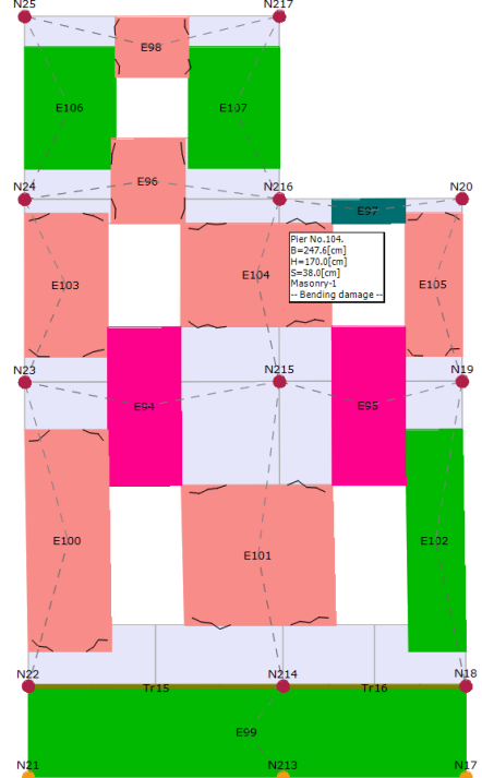
Analysis-24/Mechanism P.32 /Internal masonry /seismic dir.-Y/seismic load =static
