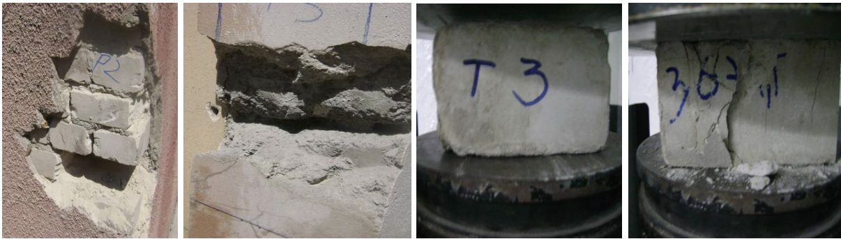
Figure 52. (a) Photo taken while sampling white brick on a perimeter wall, the eastern part from behind; (b) sample of white brick taken on the north façade wall, (c) Sample of white brick during the laboratory test in printing, (d) Sample of white brick after completion of the test in compression, at the point of destruction (Altea & geostudio, 2019)
