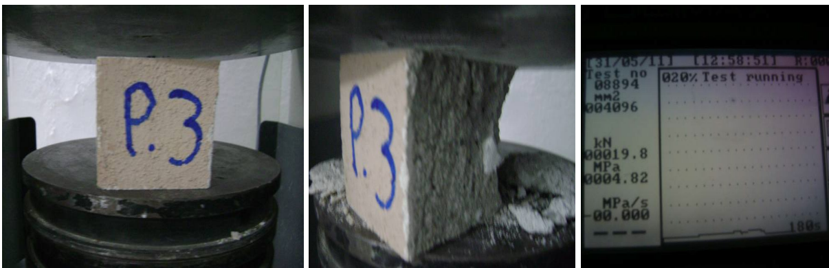
Figure 54. (a) sample of mortar during the compression test, (b) sample of mortar after completion of the test, point of collapse, (c) test result in digimax (Altea & geostudio, 2019)
