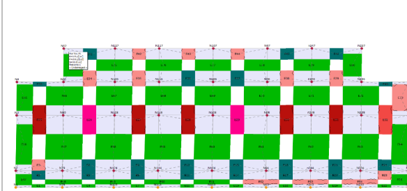
Analysis-18/Mechanism P.1 /Main façade masonry /seismic dir.+Y/seismic load =uniform
