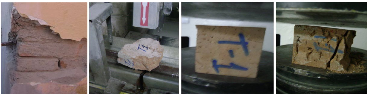
Figure 51. (a) Photo taken while sampling red brick on a perimeter wall panel, inside the basement; (b) sample of red brick preparing for laboratory test, (c) Sample of red brick during the laboratory test in printing, (d) Sample of red brick after completion of the test in compression, at the point of destruction (Altea & geostudio, 2019)
