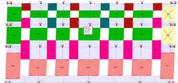
Analysis-09/Mechanism P.08 /Back façade masonry /seismic dir.+X/seismic load =uniform
