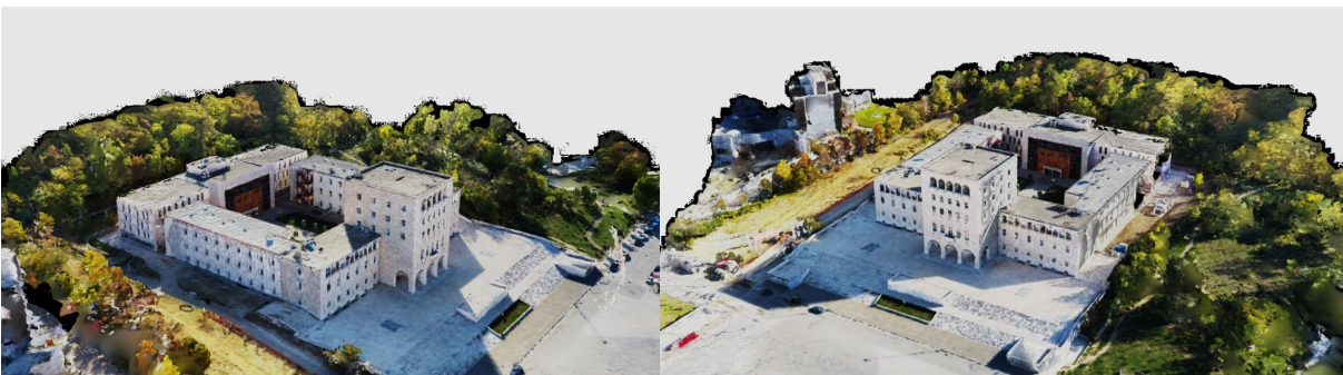
Figure 96. 3D photogrammetric model, processed after the on-site survey phase, in the framework of BIM modeling
