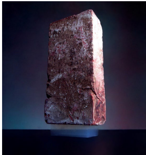
Fig. 3. Aerogel is one of the best examples of smart material thanks to its extreme lightness and strength. Source: Courtesy NASA/JPL-Caltech, Public domain, via Wikimedia Commons
