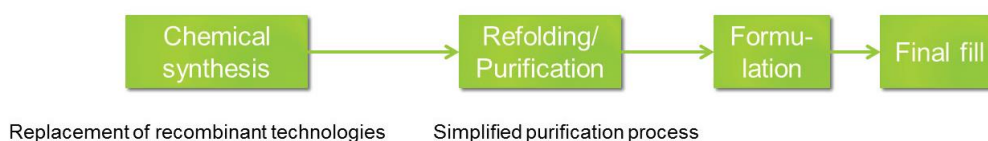
Figure 2 Comparison of manufacturing processes of a biopharmaceutical produced in cell culture to a chemically synthesized peptide. Large amounts of cell mass and cell components need to be completely removed from the biologically produced therapeutic by employing a complex set of different filtration and separation technologies (e.g. chromatography). Chemical peptide and oligos synthesis lack the high level of cell-based impurities which simplifies the purification process. [23]
