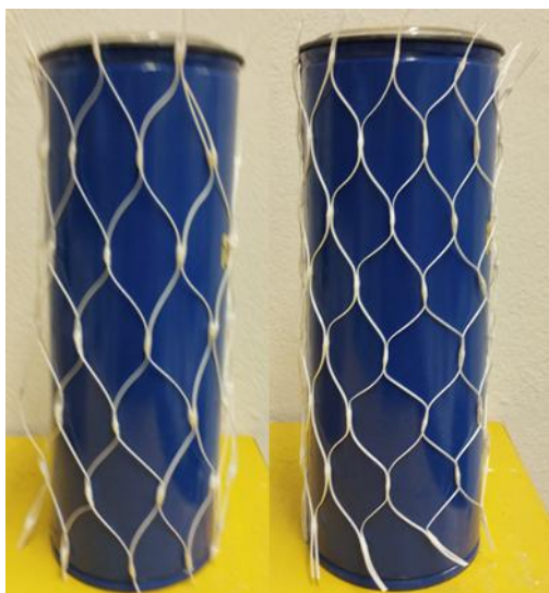
Figure 3.4 The two fabricated PLA socks, on the left the wider meshes (Sock 1), on the right the narrower meshes (Sock 2)
