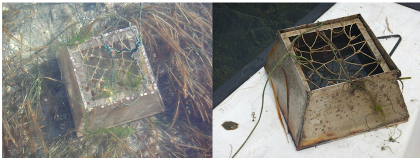
Figure 2. Sedimentation traps in Plexiglas to the left and in stainless steel to the right.
