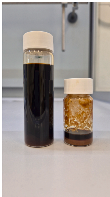
Fig. 1. Vials showing the products obtained from the solvolysis process: a) the liquid phase and b) the solid phase.
