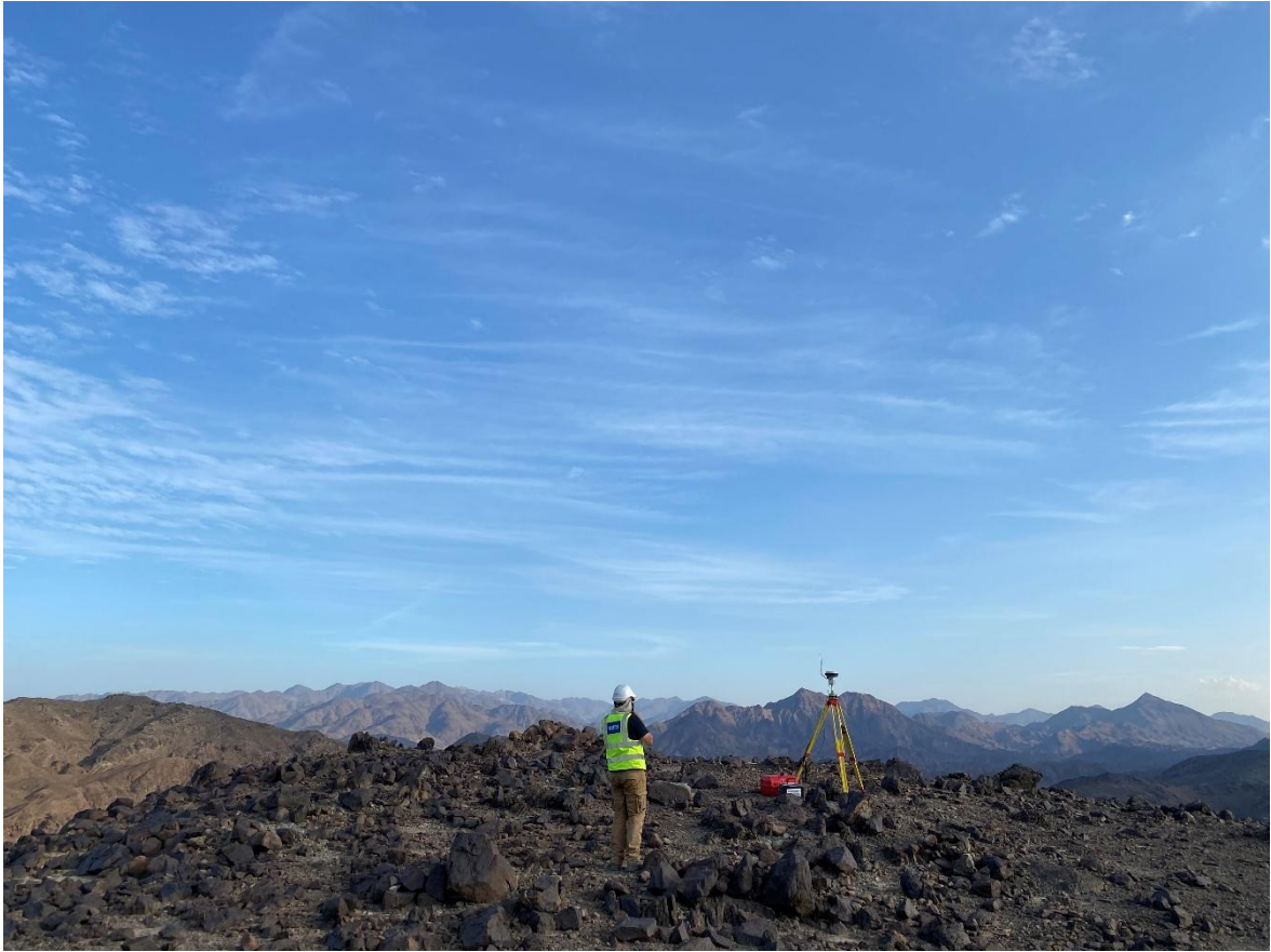
Figure 18. Leica GS15 base station setup in the UAE survey area. Installation of the Leica GS15 GNSS receiver at the highest morphologic point to ensure optimal radio link coverage with the rover GS14 during the topographic survey operations. The elevated positioning minimized signal obstruction across the rugged volcanic terrain.
