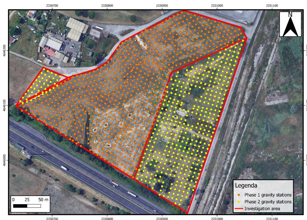
Figure 11. Orthophoto of the microgravity survey site showing the investigation area and measurement layout. Phase 1 gravity acquisition points are displayed in orange, while additional acquisition points are shown in yellow, arranged on a regular 8 \times 8 m grid covering approximately 50,000 m 2 .
