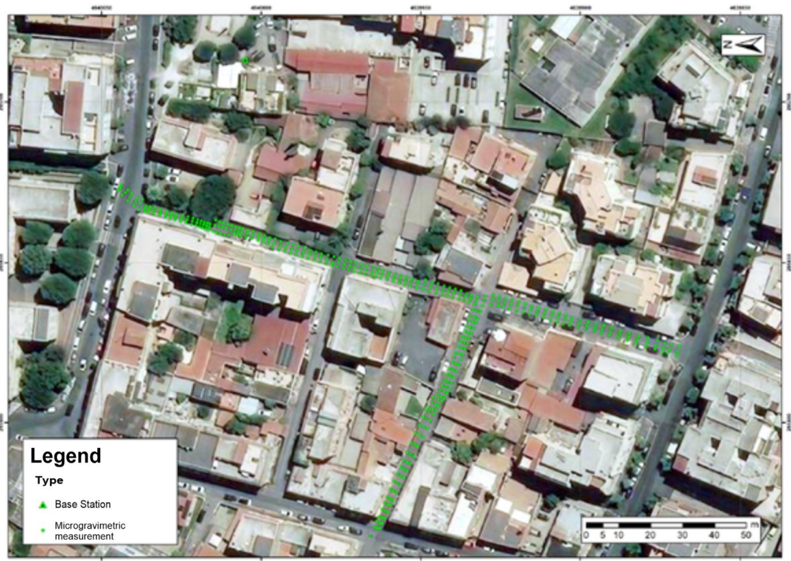
Figure 7. Survey layout of the Pigneto district, Rome. Aerial view showing the microgravity measurement network and base station locations along the urban streets of the Pigneto area. The survey design follows the main road intersections to maximize spatial coverage and detect potential subsurface anomalies related to sinkhole susceptibility beneath the built environment.
