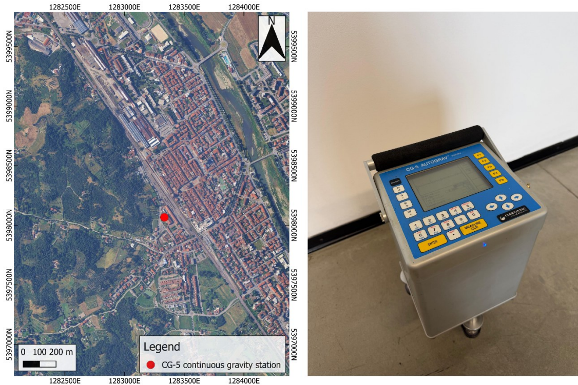
Figure 35. Location of the CG-5 continuous gravity station at the Centro di Geotecnologie, San Giovanni Valdarno, and photograph of the instrument setup during laboratory acquisition.
