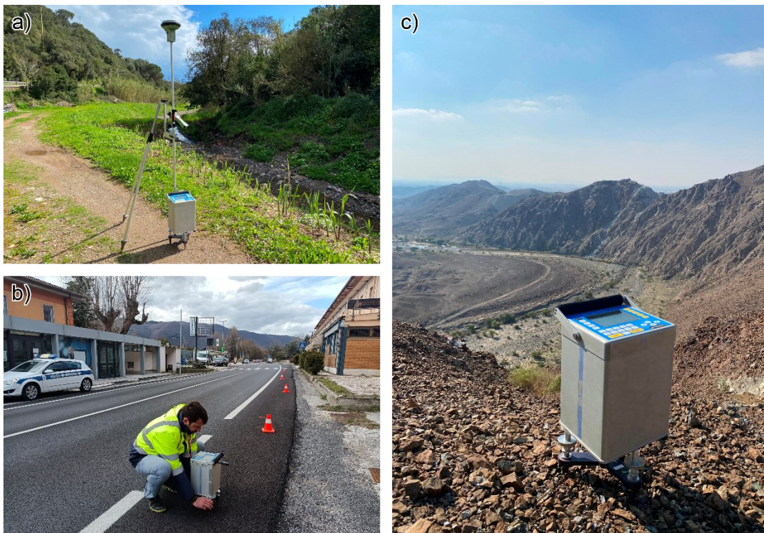
Figure 38. Scintrex CG-5 gravimeter in different survey environments: (a) installation along a vegetated rural path, (b) data acquisition in a roadside urban setting, and (c) deployment on steep rocky terrain within a mountainous desert landscape.
