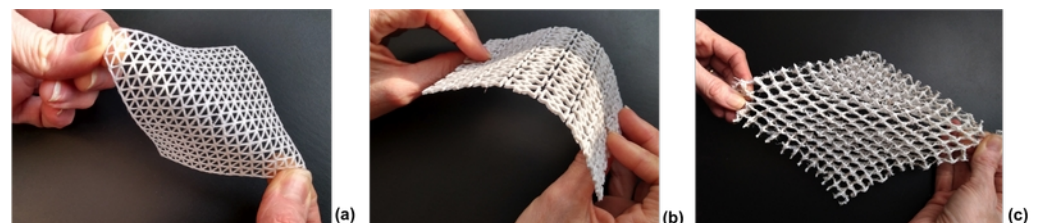
Figure 4. filter printed in PLA / PCL: (a): dimensional stability (b) flexibility (c) dimensional stability.
