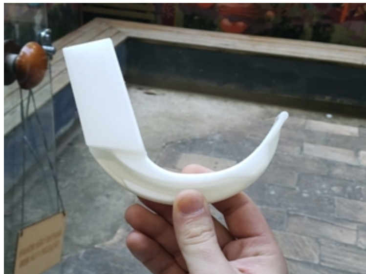
Figure 5 - Video laryngoscope model developed by the DAD-PUC-Rio team based on the Air Angel setup. (source: authors)
