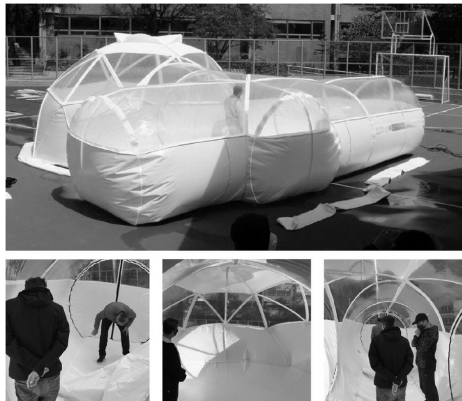
Figure 20. One-to-one scale prototype of the basic construction module of the system.
