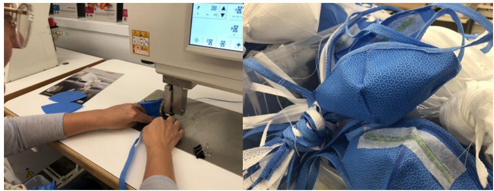
Figure 9 Ultrasonic Welding for Dome Disposable Masks
