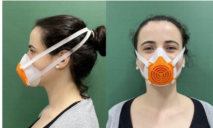
Figure 4 - DAD-PUC-Rio Team member using the under development TPU/PLA 3D printed N95 prototype. (source: authors)
