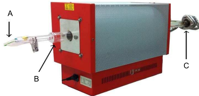
Figure 1.4: Hot wall furnace used for graphene synthesis. (A) indicates the port where gases are introduced, (B) is the quartz tube where the copper foil is placed, (C) is the furnace connection to the vacuum pump and way-out connection for exhaust gases.
