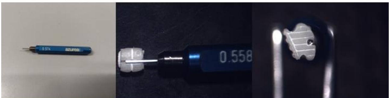
Figure 2. Azurea pin gauges (Azur a Technologies S.A., Switzerland) and the microscopic image of the gauge inserted in the bottom of the slot.
